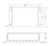
$\begin{array}{ll} \text{1.The size of SR-DH100} & \text{is as follows:} \\ \text{Boundary dimension:} & 82\times100\times20 (\text{mm}) \\ \text{Installation dimension:} & 86\times75 (\text{mm}) \\ \text{Installation aperture:} & 3.5 (\text{mm}) \\ \text{2.The size of SR-DH50} & \text{and SR-DH20:} \\ \text{Boundary dimension:} & 82\times58\times20 (\text{mm}) \\ \text{Installation dimension:} & 43\times75 (\text{mm}) \\ \text{Installation aperture:} & 3.5 (\text{mm}) \\ \end{array}$
