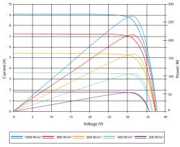
Excellent performance under weak light conditions: at an irradiation intensity of 200 W/m² (AM 1.5, 25 °C), **96.5%** or higher of the STC efficiency (1000 W/m<sup>2</sup>) is achieved
